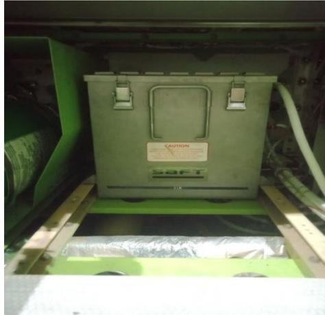
Gambar 1. Baterai Dari Electronic Equipment Compartment
