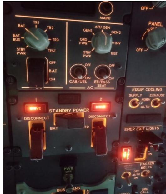
Gambar 4. Standby Power Switch
