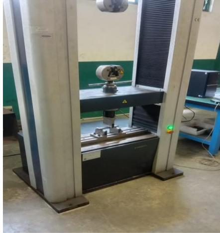
Gambar 2. Mesin Uji Bending Universal
