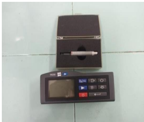
Gambar 1. Alat Uji Surface Roughness Tester
