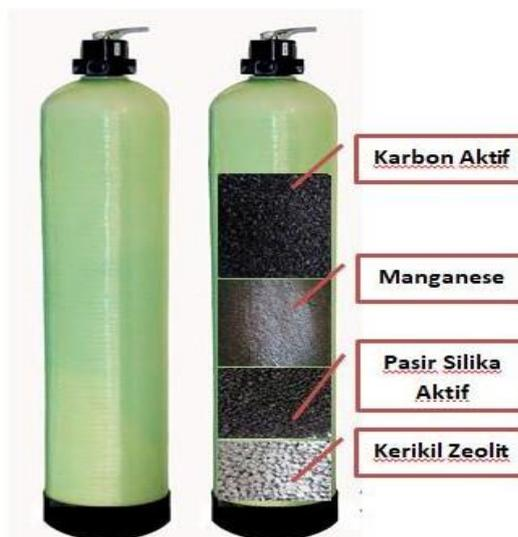
Gambar 3. Penampang filter dan susunan media filter
